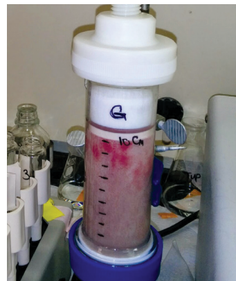
Activator test column showing mobilized NAPL (dyed red). Courtesy of Tufts University
